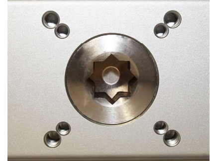
Bottom mounting conforms to ISO5211 and DIN3337. Models PDC32 and PDC190 to PDC300 have 1 bolt pattern, all others have 2.
